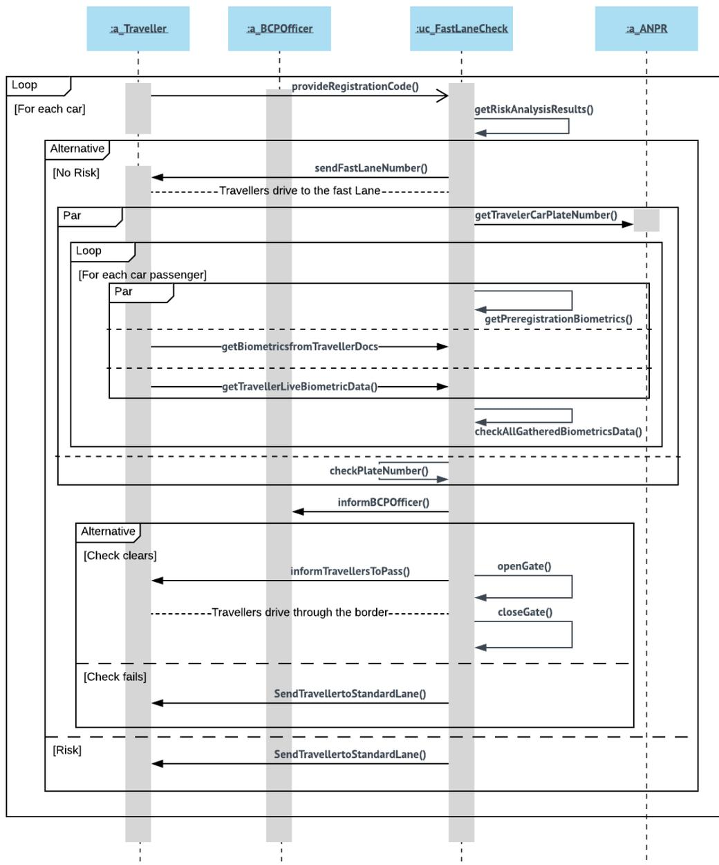
Figure 5 Fast lane check system - use case scenarios diagram: Vehicle Scenarios
