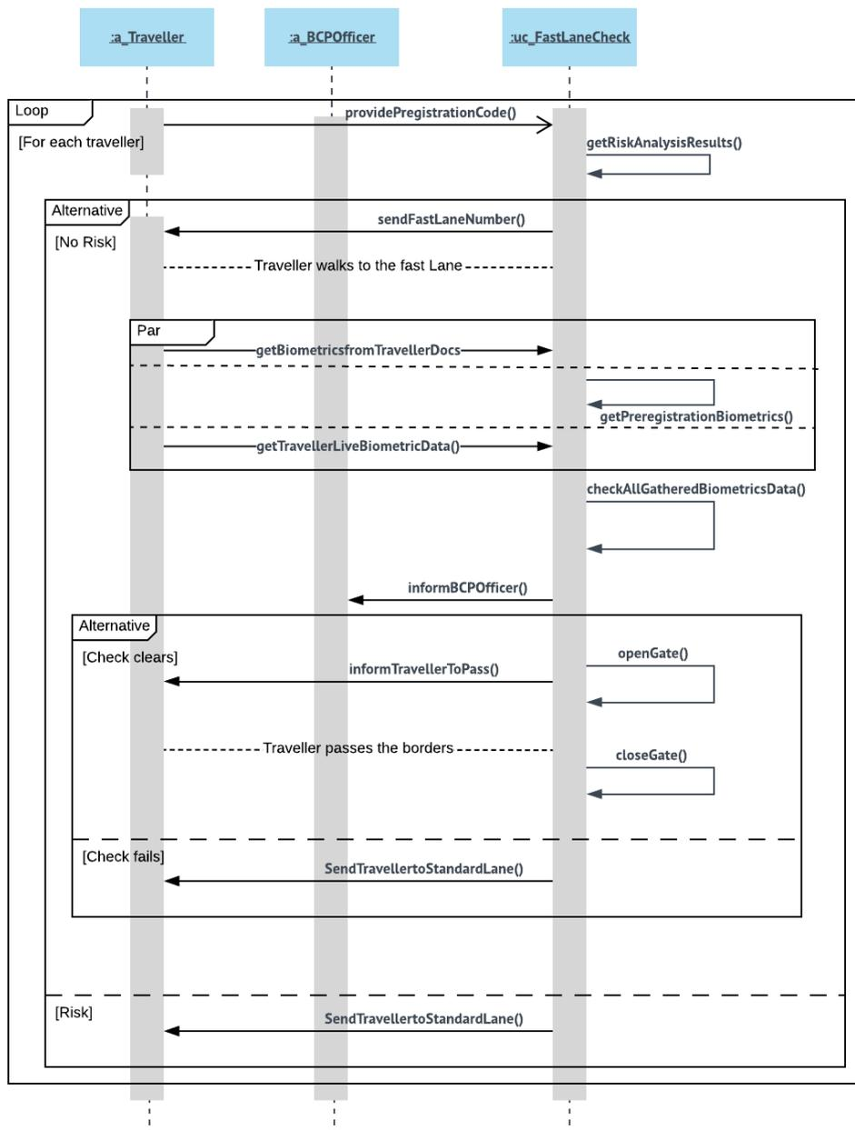
Figure 4 Fast lane check system use case scenarios diagram: Pedestrian Scenarios
