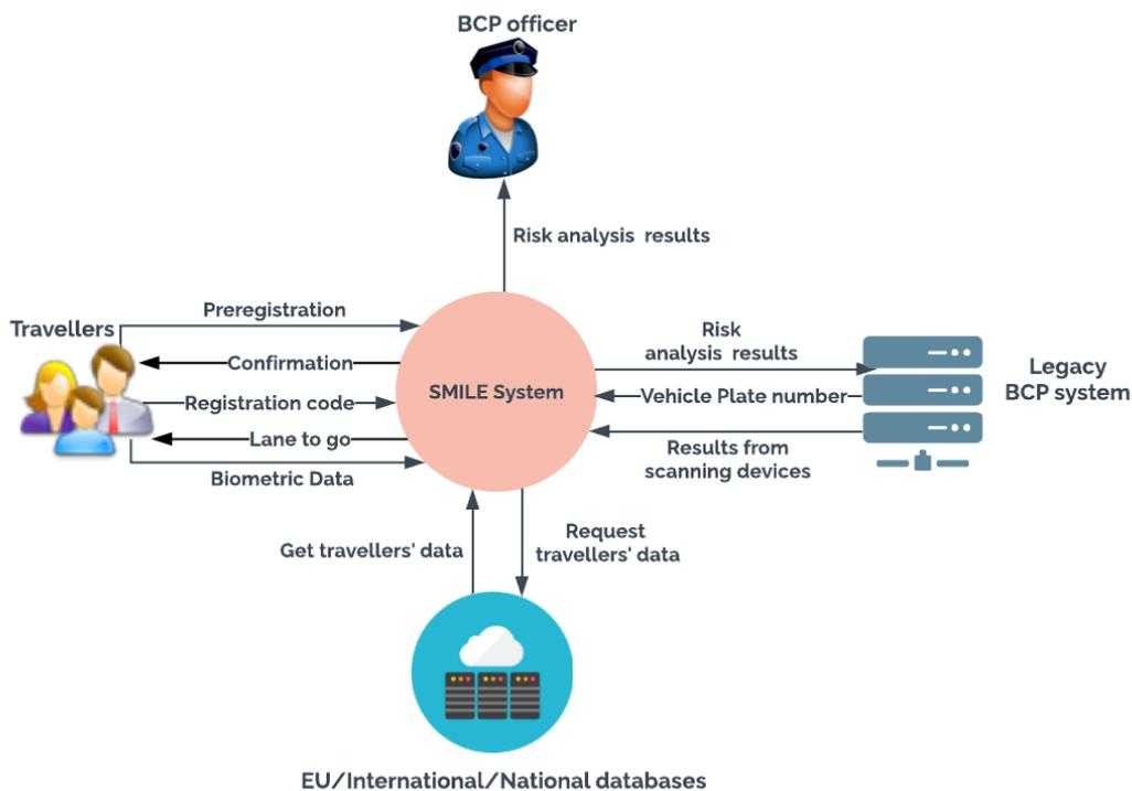
**Figure 1 SMILE's system scope diagram**
