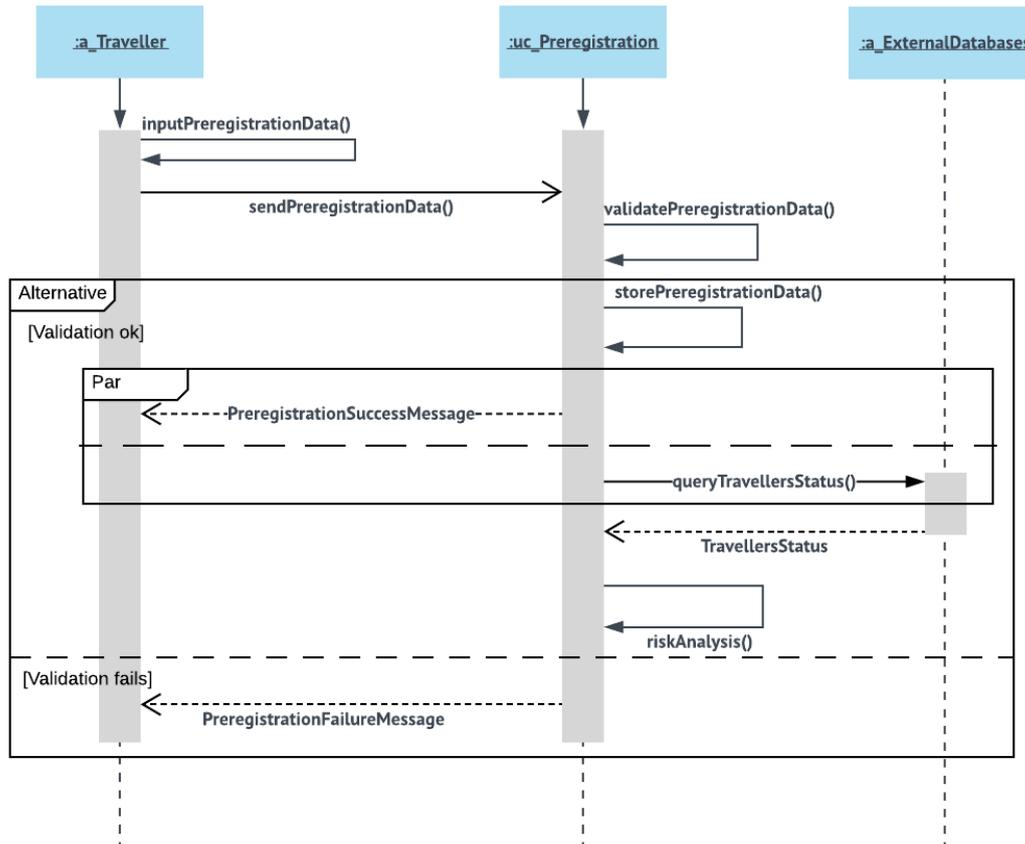
Figure 3 Preregistration – system use case scenarios diagram
